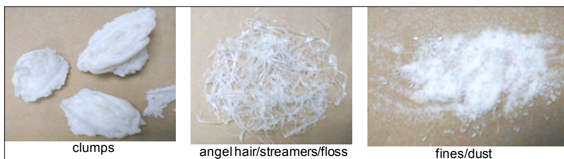
Figure 3.3 Types of degradation in delivery/conveying
