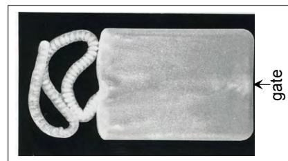
Figure 3.10 Short-shot moulding showing jetting (source: Akay (1992))
