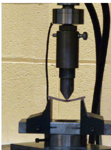
Figure 6.14 A specimen tested in 3-point bending
