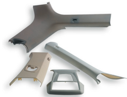
Figure 6.48 Molded part: textile is back injected (Source: Georg Kaufmann Formenbau)
