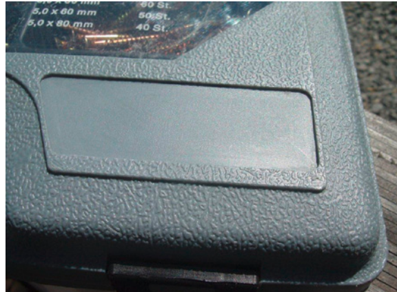
Figure 7.2 Molded part with graining (Source: Willi Haller)
