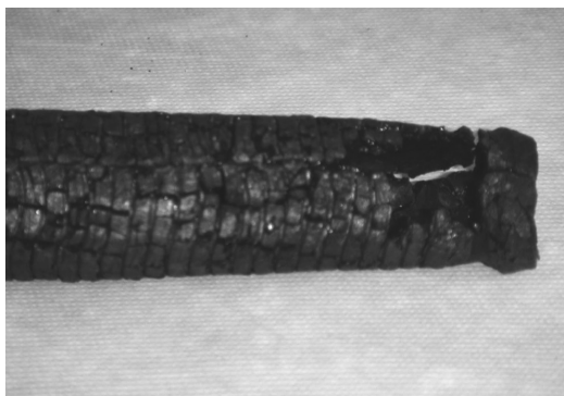
Figure 2.2 Golf grip severely degraded by its brass-colored coating
