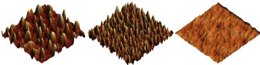
Figure 2.5 Atomic force microscopy images ( 2 \times 2 \mu\text{m} ) of acrylic acid plasma polymers after 60 s (left), 90 s (middle) and 240 s (right), showing initial island formation followed by island intergrowth, eventually resulting in a smooth film. The height scale is the same for each image, with a maximum peak height of 10.9 nm.
