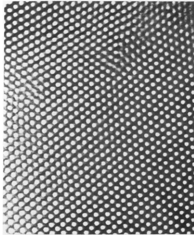
FIGURE 2.4 Transmission electron photomicrograph of an ultrathin film of a styrene-isoprene-styrene triblock copolymer (MW 16,200–75,600–16,200) \times 100,000 .
