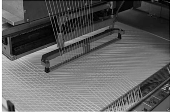
Fig. 7.13 Magazine weft insertion of the Karl Mayer Malitronic® Multiaxial stitch-bonding machine
