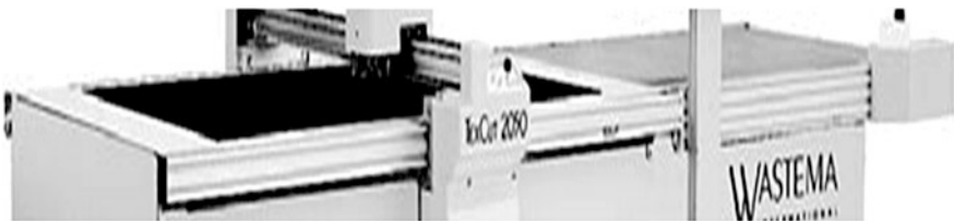
Fig. 12.9 CNC cutter with stitch knife [9] (Source: Wastema International Steinhauser Spezialmaschinen GmbH)
