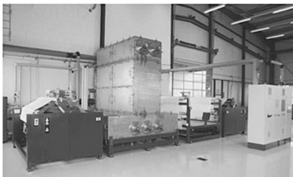
Fig. 13.38 Fluorine treatment in continuous processing ( Source: Fluor Technik System GmbH )
