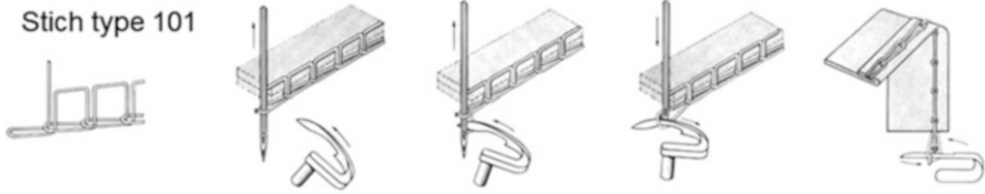
Fig. 12.11 Single chain stitch formation principle [12] (Source: Pfaff Industriesysteme und Maschinen AG)
