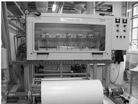
Fig. 13.35 Corona/plasma unit by Ahlbrandt, with gas input and atomizing system for pretreatment of textile materials under atmospheric pressure
