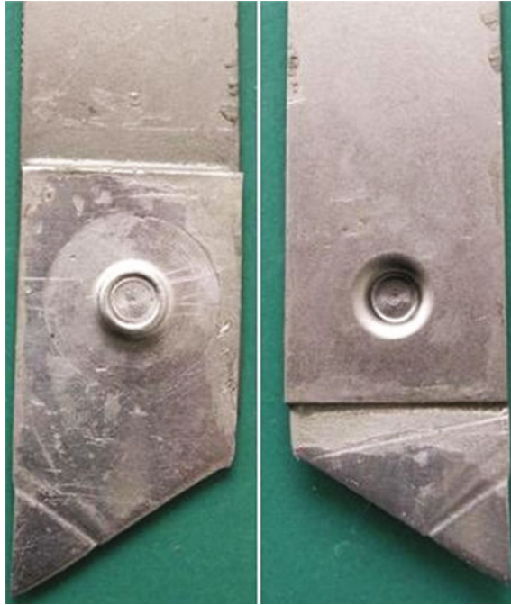
Fig. 46 Hybrid clinch-adhesive joint of aluminium sheets after pull test
