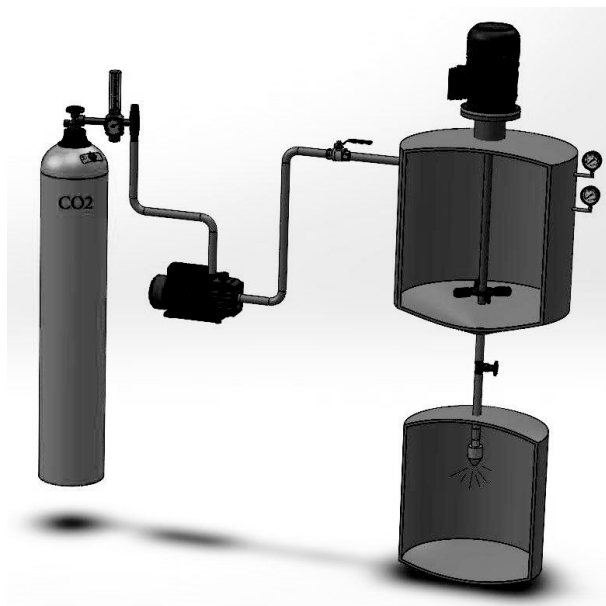
Figure 7.2 The particles from gas-saturated solution (PGSS) technique.
