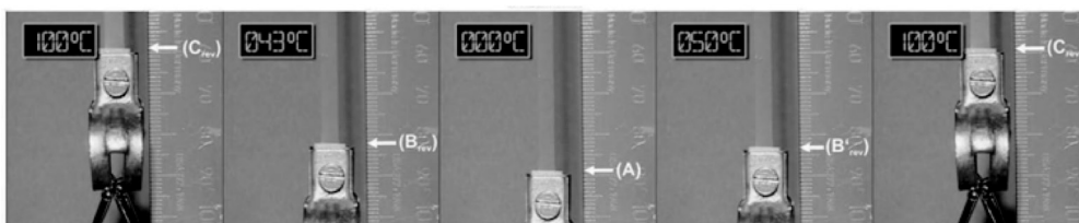
Figure 2.8 Examples of reversible shape-memory behaviour. Reproduced with permission from J. Zotzmann, M. Behl, D. Hofmann and A. Lendlein, Advanced Materials , 2010, 22 , 31, 3424. ©2010, John Wiley & Sons [66]
