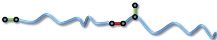
Figure 8.1 Possible positioning of mechanophores: chain end, side chain, and chain center. Activation is highest when the mechanophore is at the chain center and the polymer chain passes through both ends of the activated bond.
