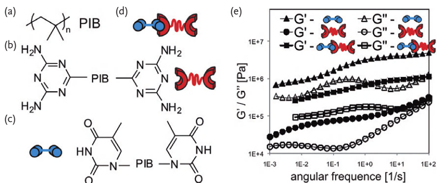
Figure 11.10 (a) Structure of supramolecular polyisobutylene (PIB); (b) PIB bearing 2,6-diaminotriazine groups; (c) PIB bearing thymine groups; (d) equimolar mixture of PIB-Thy and PIB-DAT; (e) frequency sweep
