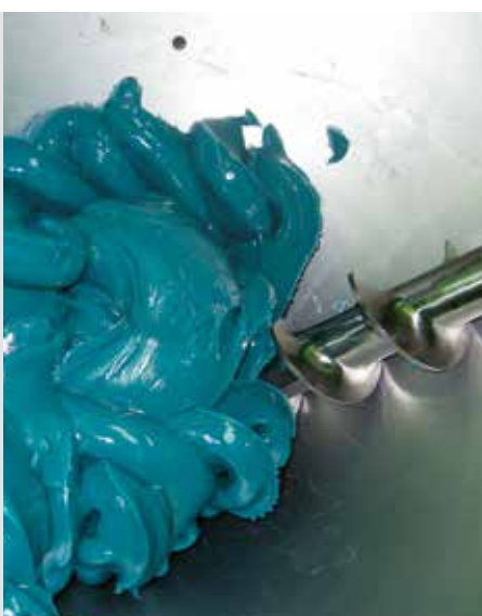
Interior of the RotoFeeder®: Feed hopper with conveying screw
