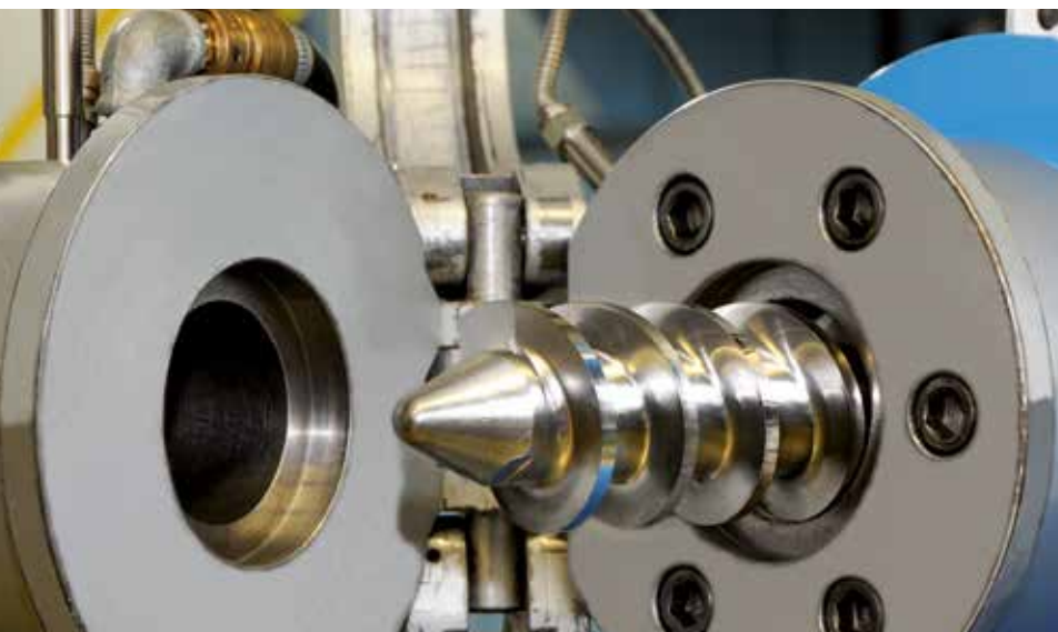
Open extruder with conveying screw
