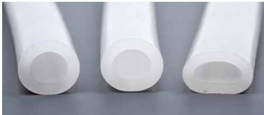
Fluctuations in the extrudate geometry
