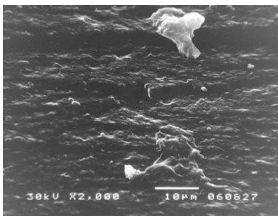
Fig. 9.23 SEM micrograph with magnification X = 2000 of NBR/EPDM composite containing 70 phr CB
