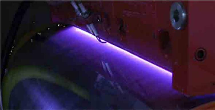
**Figure 12.1** Flame treatment equipment developed to activate webs or polymeric films. The common configuration for this type of activation is roll to roll.
