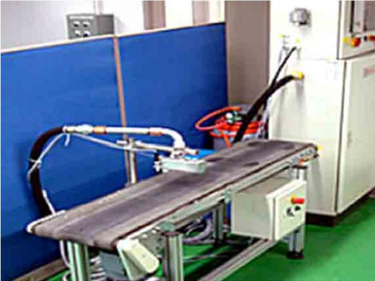
**Figure 12.4** Flame treatment equipment able to activate 2D plastic parts. The components slide under the flame and only one side of the component is surface activated.
