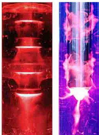
**Figure 10.2** Cavitation phenomenon occurring during ultrasonication in two differently shaped probes [42]
