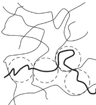
FIGURE 3.2 Subdivision of a chain into blobs in semi-dilute solutions.
