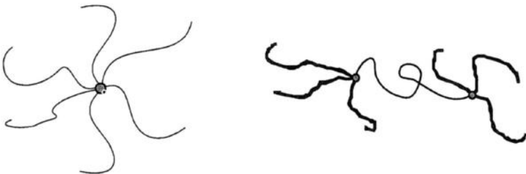
FIGURE 7.15 Schematic of a six-arm star polymer (left) and a multiarm branched polymer (right).
