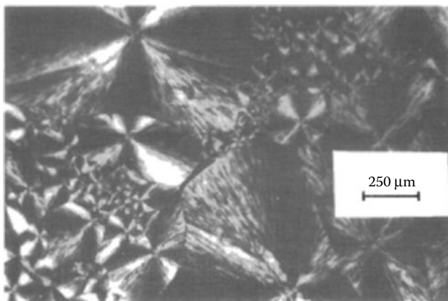
FIGURE 3.16 Spherulitic structure of poly(ethylene oxide) seen between crossed polarizing sheets.
