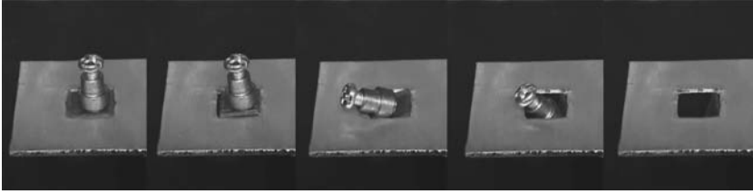
FIGURE 1.10 SMP for automatic hole opening upon heating.
