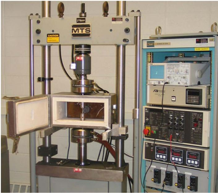
**Fig. 5.6** Closed-loop servo-controlled hydraulic testing system
