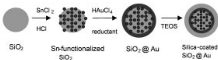
15.5 Schematic diagram for the synthesis of gold-coated silica nanoparticles.
