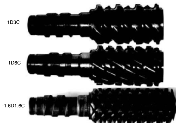
Figure 10.36: Rhomboidal mixing sections studied experimentally.
