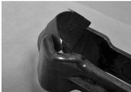
FIGURE 8.9 Flexible MWNT/HEC-PAAm nanocomposite aerogel prepared by deposition of nanotubes on to the preformed polymer gel.
