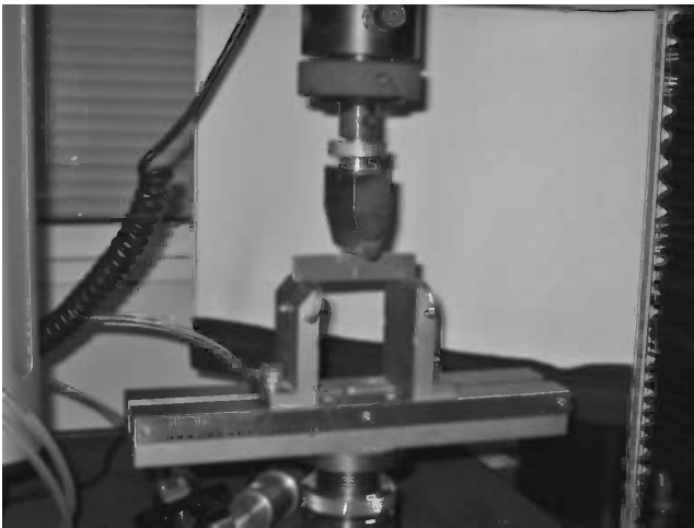
FIGURE 2.1 Typical test setup of a three-point bending test of SENB specimen.
