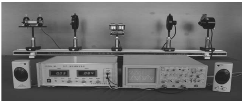
Figure 2.21 The setup of a commercially available magneto-optical isolator.
