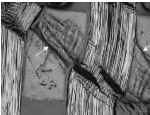
Figure 13.29 Matrix cracks in the transverse yarns (arrows) due to the lateral pushing by the fractured axial yarns.
