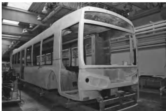
Figure 23.2 NABI composite bus shell production by Seemann Composites Resin Infusion Molding Process (SCRIMP) [12].
