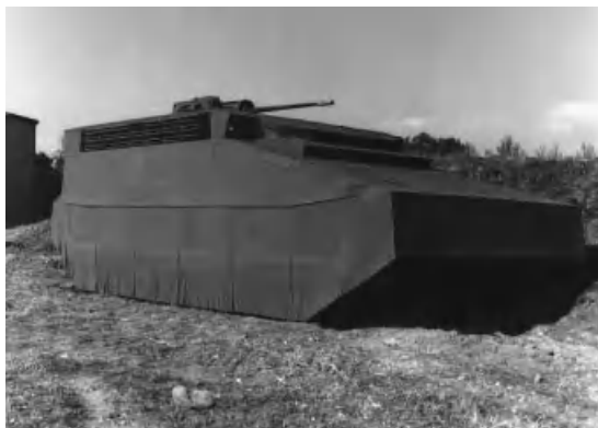
Figure 23.18 Composite Armored Vehicle made of S-2 Glass Fiber Rovings by vacuum-assisted resin transfer molding (VARTM) technology [147].
