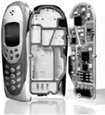
Figure 23.12 EMI shielding gaskets made from metal particle loaded elastomeric polymers used in several applications.
