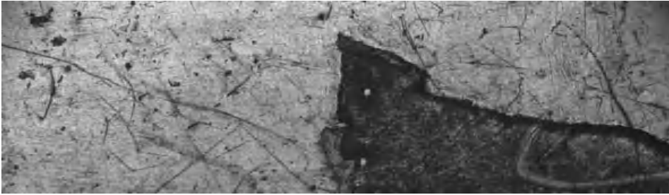
Figure 16.21 Micrograph of the area at the interface between conductive and nonconductive surface of a Vestamid LR1-MHI component molded at a constant screw feed rate of 50 mm/s.
