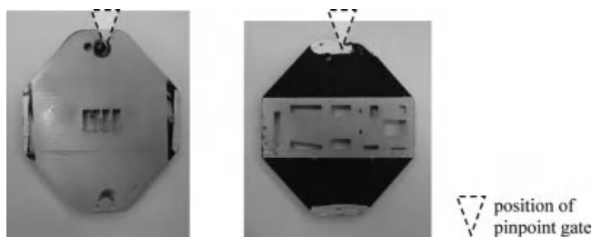
Figure 16.24 Galvanic starting tests on completely filled components with different geometries.
