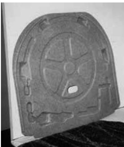
Figure 5.2 PLA compound material parts reinforced with kenaf fiber.
