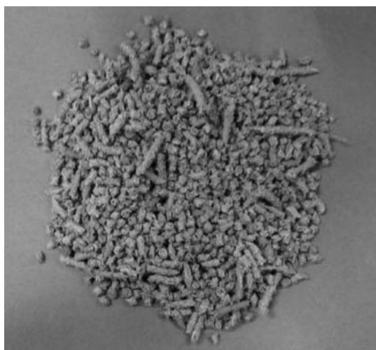
Figure 5.14 Bamboo fiber reinforced thermo plastics (BF RTP) manufactured using roller materials.
