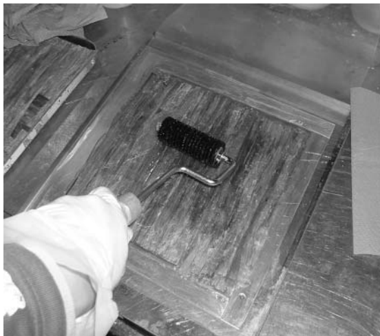
Figure 6.1 Lab-scale fabrication of multi-ply, unidirectional kenaf, and fiber-reinforced ortho-UP composites by hand layup [12].
