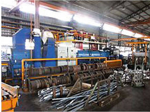
Fig. 5.3 A horizontal hydraulic press for hot aluminum extrusion (loose dies and scrap visible in foreground)
