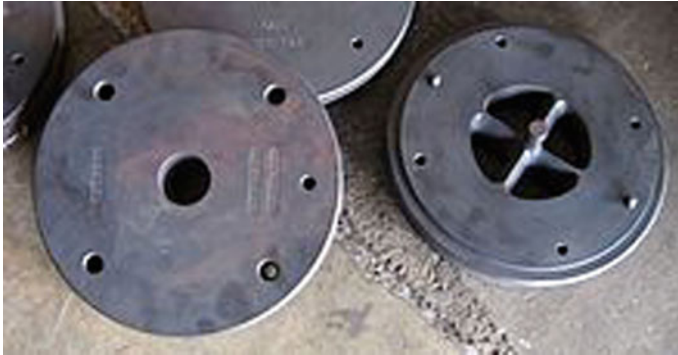
Fig. 5.4 Two-piece aluminum extrusion die set (parts shown separated). The male part (at right ) is for forming the internal cavity in the resulting round tube extrusion
