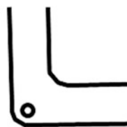
Fig. 3.21 Design features to avoid the effects of sharp corners
