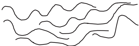
Figure 2.3 Schematic structure of a thermoplastic.
