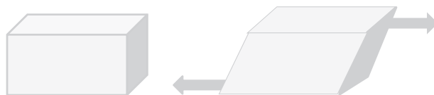
Figure 7.3 Example of in-plan shear deformation.
