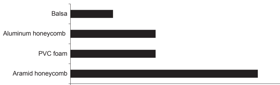
Figure 3.15 Relative costs of various cores for sandwich composites.
