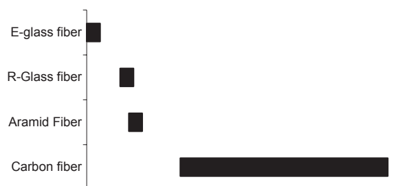
Figure 3.14 Relative costs of various fiber reinforcements.
