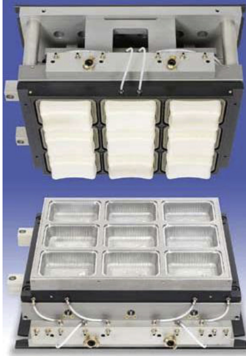
Figure 6.1 An example of plugs made of syntactic foams used in thermoforming. Images courtesy Jeff Barker, Tooling Technology LLC, Fort Loramie, OH.
