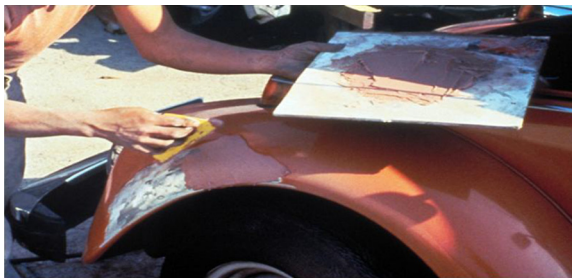
Figure 9.1 Auto repair compound being applied to a sheet metal of automobile bodies.
