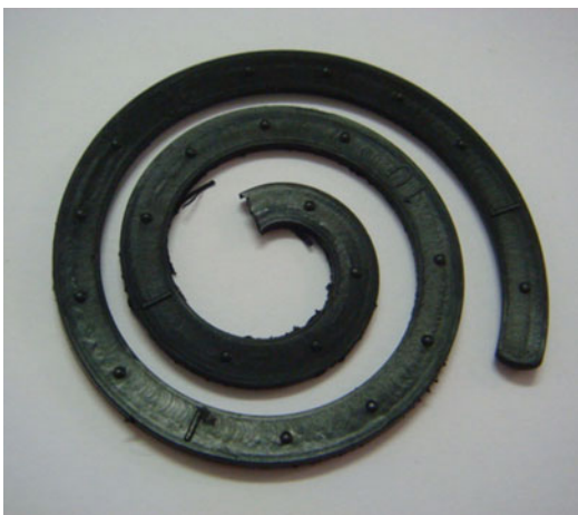
Fig. 19.11 Elastomer sample after vulcanization in the helix test
