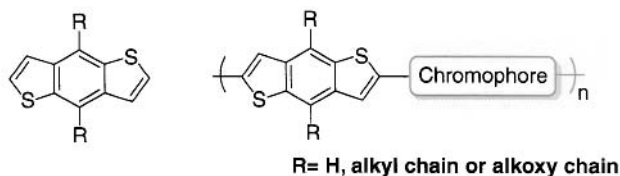
Scheme 3.1 General structures of benzo[1,2- b :4,5- b' ]dithiophene (BDT) unit (left) and BDT based copolymers (right).
