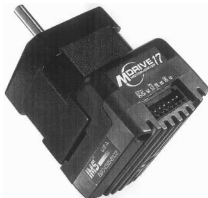
Figure 5.1 Thermally conductive carbon fiber-reinforced PPS injection molded stepper motor enclosure—heat sink. (Courtesy of Cool Polymers, Inc.)
