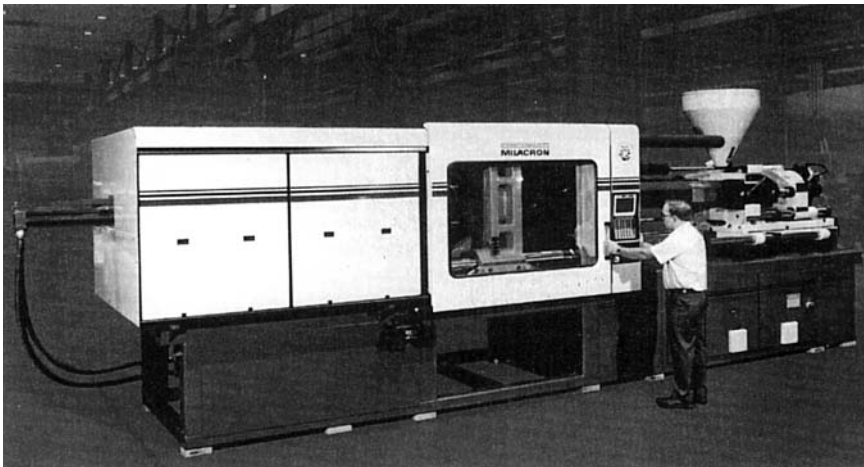
Figure 9.11 Model VT550 550-ton toggle-type injection molding machine. (Photo provided by Cincinnati Milacron, Inc.)
