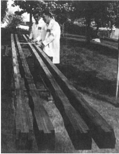
Figure 4.24 Filament-wound/protruded graphite epoxy bridge beam. (Courtesy of Sci. Div. of Harsco)
