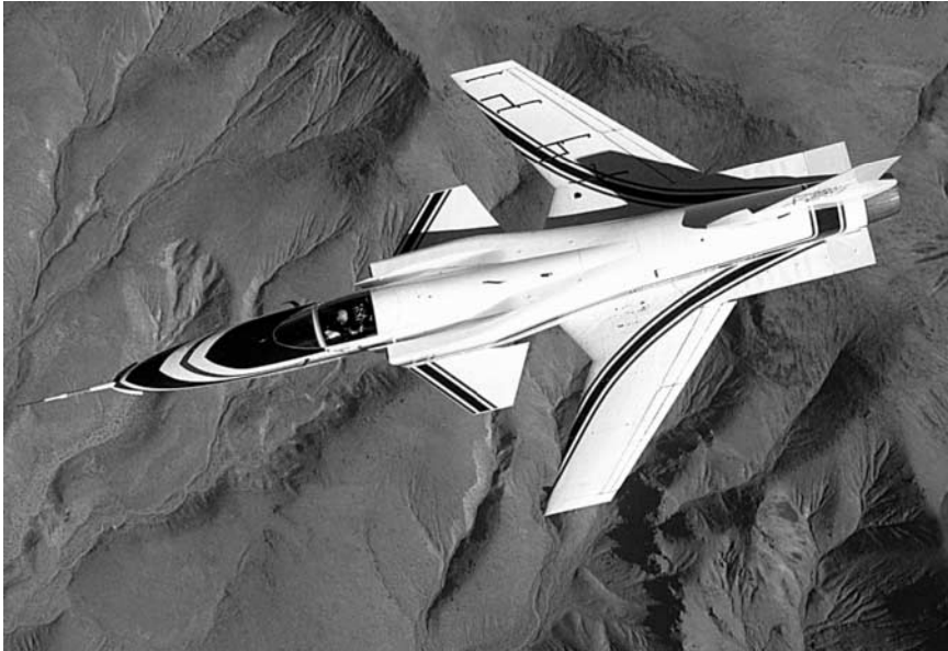
Figure 4.3 NASA-Grumman forward-swept wing, X-29 aircraft. (Courtesy of Dryden Flight Research Center)
