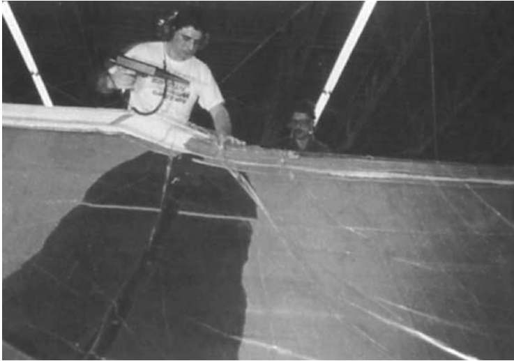
Figure 4.17 RTM (SCRIMP™) process for injecting a boat hull. (Copyright Billy Black, courtesy of Seemann Composites)
