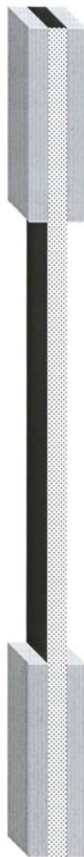
Figure 6.6 A representation of tabbed specimens used for tensile testing of fibre-reinforced composites
