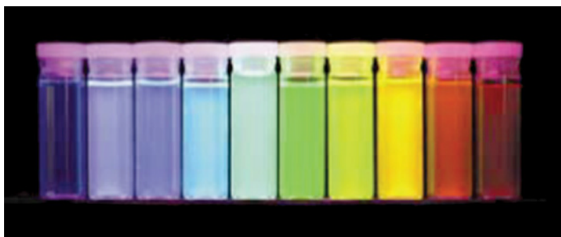
Figure 7.2 Light emission of ZnS-capped CdSe excited in the UV range. Dimension of colloidal QDs increase from 2 (left) to 6 (right) nm. Chan et al. [10]. Reproduced with permission of Elsevier (See insert for color representation of the figure)
