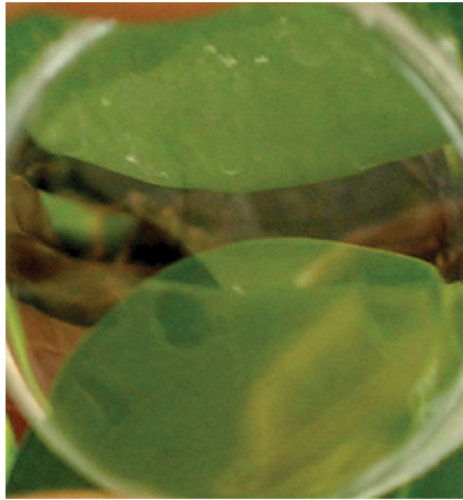
Figure 7.18 PS/PMMA polymer blend containing 5% ZnO Nanoparticles. Ge et al. [135]. Reproduced with permission of Wiley
