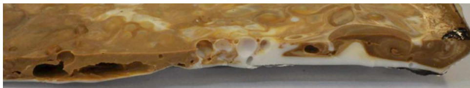
Figure 9.3 Cross-section picture of polyethylene terephthalate residue obtained by interrupted combustion just after TTI. Fina and Camino [13]. Reproduced with permission of Wiley (See insert for color representation of the figure)
