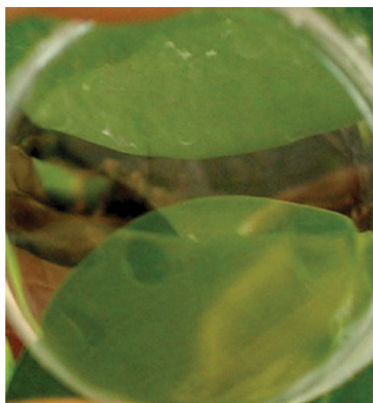
Figure 7.18 PS/PMMA polymer blend containing 5% ZnO Nanoparticles. Ge et al. [135]. Reproduced with permission of Wiley (See insert for color representation of the figure)
