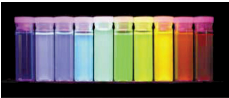
Figure 7.2 Light emission of ZnS-capped CdSe excited in the UV range. Dimension of colloidal QDs increase from 2 (left) to 6 (right) nm. Chan et al. [10]. Reproduced with permission of Elsevier
