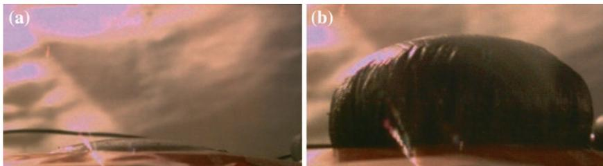
**Fig. 10** Actuation of ACM rubber IPN plasticized with 40 wt% DBEF at  $-40$  C, **a** voltage off, **b** voltage on, 6.5 kV (215 % areal strain) [17]. Copyright 2010. Reproduced with permission from John Wiley & Sons
