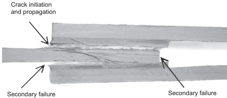
Figure 3.3 Failure mode of adhesively-bonded GFRP joint under tensile loading.
