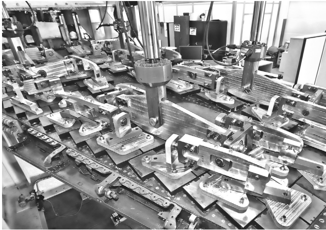
Figure 10.19 Four-actuator tension–compression whiffletree over wing.
