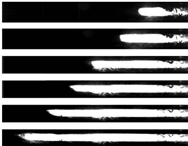
Figure 6 Sequential images of the flame propagating along the tube.
