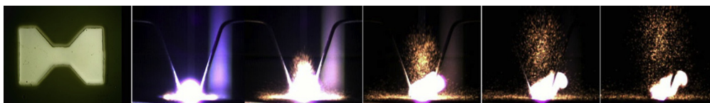
Figure 21 Al/Ti multilayer bridge and its electrical explosion at 100 cycles, capacity 100 \mu F, and charge voltage 140 V.
