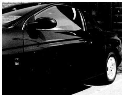
FIG. 9 Example of PC/ABS used in body panels: Saturn PC/ABS door panels.
