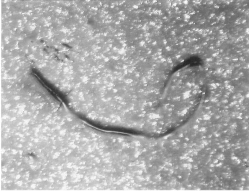
FIG. 14 Dirt—an example of a fiber.
