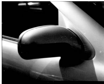
FIG. 15 Example of PPO/PA used in mirror housing: 2000 Mercedes CL500 mirror housing.
