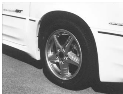
FIG. 8 Example of PC/ABS used in wheel covers: Pontiac Grand AM GT.
