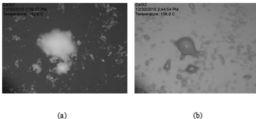
FIGURE 18.7 Optical micrographs of \text{CaSt}_2 powder at: (a) 142.8^\circ\text{C} , and (b) 156.6^\circ\text{C} .
