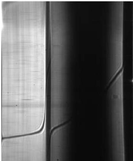
**Figure 12.8** Schlieren image of the hybrid latex containing polyurethane encapsulated pigment particles (density gradients, after 22 h at 40000 rpm, 25 °C, 20 wt% nycodenz in water). The first band shows the free polymer (density  $1.066 \text{ g cm}^{-3}$ ), whereas the second broad band (density  $1.083\text{--}1.165 \text{ g cm}^{-3}$ ) indicates the encapsulated pigment. Reproduced from reference [31] with permission from Springer.
