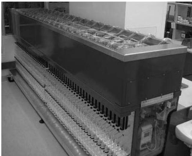
**Figure 13.1** Custom-built respirometer used by Commonwealth Scientific Industrial Research Organization (CSIRO), Australia.
