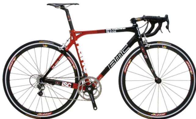
FIGURE 7.5 Bicycle with frame made of carbon nanotubes. CNTs make the bike lighter and with a high mechanical resistance.
