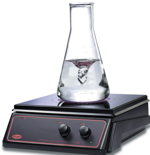
FIGURE 6.5 A stir bar mixing a solution in a magnetic stirrer with coupled heating.
