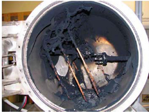
FIGURE 4.2 Lab arc discharge system for single-walled carbon nanotubes (SWCNTs) production.
