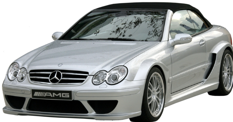
FIGURE 2.21 Numerous body components of the Mercedes CLK Cabriolet are made of carbon fiber composite material, including the luggage compartment, doors, front wings, rear wheel arches flaring, the front and rear aprons, as well as the rear airfoil.
