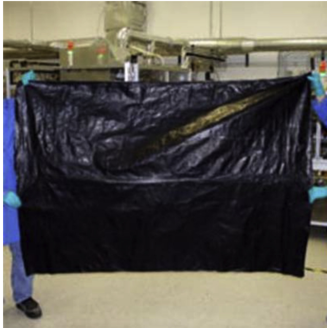
FIGURE 7.20 Large-format carbon nanotube textiles which could be used for electromagnetic interference shielding.
