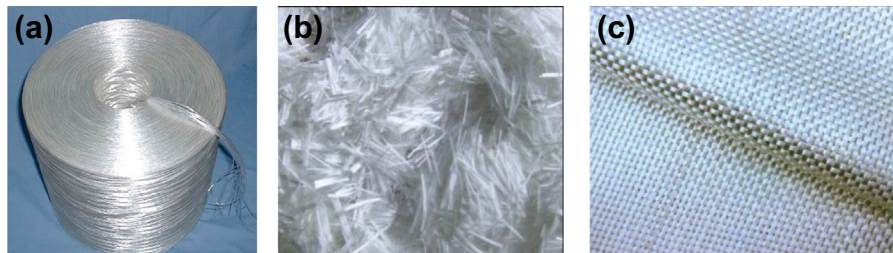
FIGURE 2.13 Glass fibers are marketed in the form of rolled continuous fibers (a), short fibers (b), and blankets (c).
