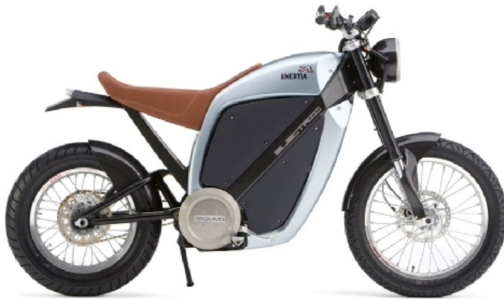
FIGURE 2.22 Enertia is an electric bike with a frame reinforced with carbon fibers.
