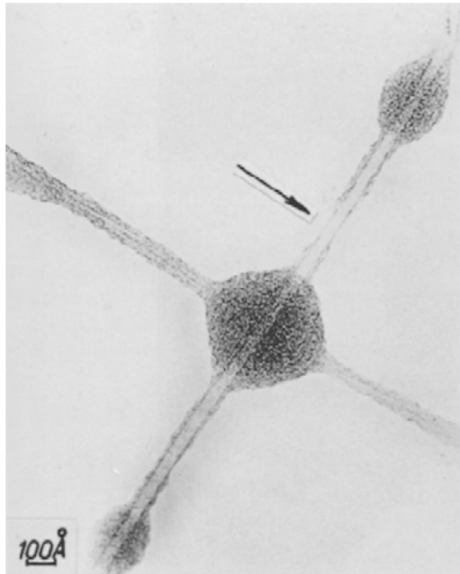
FIGURE 3.3 One of the first micrographs depicting a single-walled carbon nanotube or double-walled carbon nanotube.
