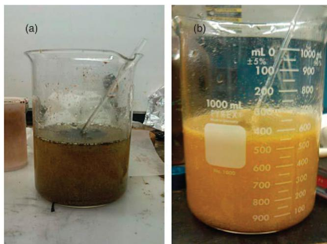
**Figure 9.5** (a) Pressurized oxidation method and (b) modified pressurized oxidation method [59].
