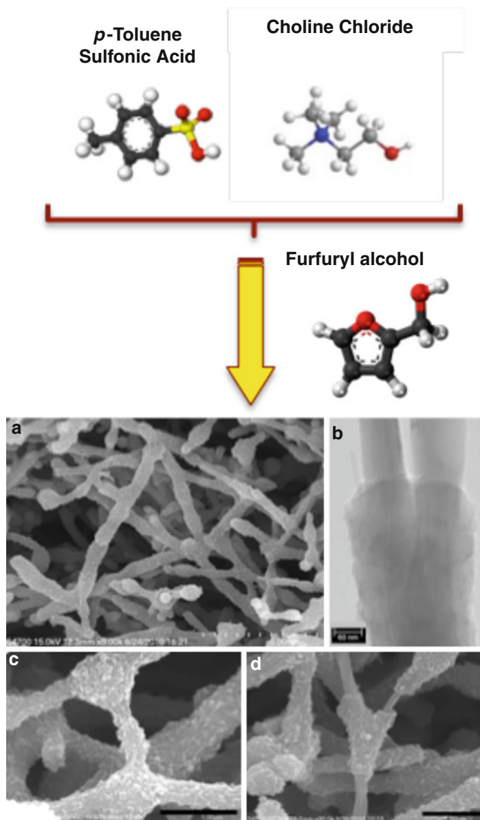
Fig. 2.4 Scheme representing the catalytic condensation of furfuryl alcohol by the eutectic mixture of p -toluene sulfonic acid and ChCl for the formation, after carbonization, of carbon-carbon nanotube composites. SEM ( a , c and d ; scale bars: 5, 1 and 1 \mu\text{m} , respectively) and TEM ( b , scale bar: 50 nm) micrographs show the hierarchical structure of the resulting monoliths (Adapted with permission from Ref. [55])
