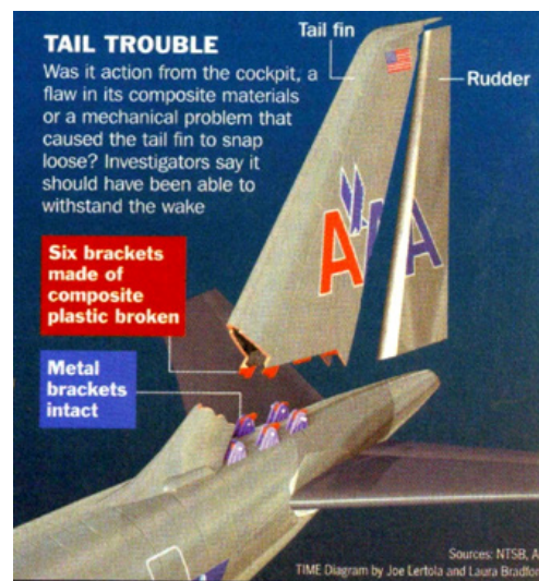
Figure 4.22 Illustration of the aircraft tail section failure at the November 2001 crash (source: TIME, November 26, 2001)
