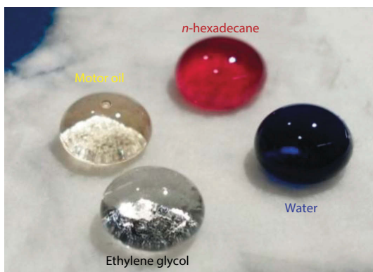
Figure 14.6 Droplets of four test liquids (water, dyed blue), ethylene glycol, motor oil, and n-hexadecane (dyed red) positioned on the handsheet depicted in Figure 14.5c; high ( >150^\circ ) contact angles are evident for all liquids. Reproduced from Ref. 39 with permission from The American Chemical Society.
