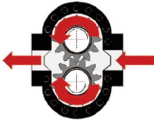
Fig. 18 Compact rubber extruder with gear pump
