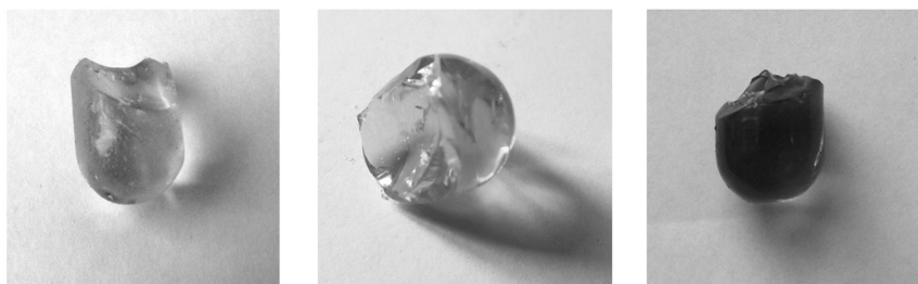
FIGURE 7.23 Samples of CL/BA = 60/40 vol%, Imidazole/BA = 70/30 vol%, and PEPA/BA = 45/55 vol% (Temperature of Syntheses 250, 220, and 150^{\circ}\text{C} , Respectively, 3 h).
