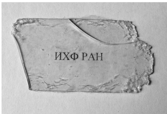
FIGURE 7.22 Cured Hybrid Resin ( T = 120^\circ\text{C} , 30 min); Plate is 2 mm Thick. The Signature is Located Under the Plate.
