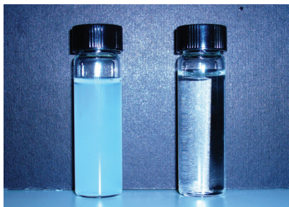
Fig. 2. CHAp nanoemulsion (left) as compared to pure water (right).
