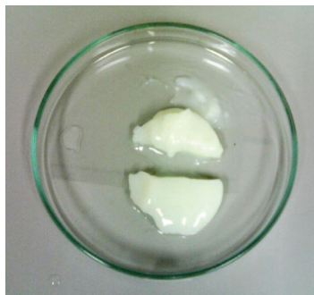
Fig. 3. As-synthesized wet slurry nanoparticles before freeze-drying.
