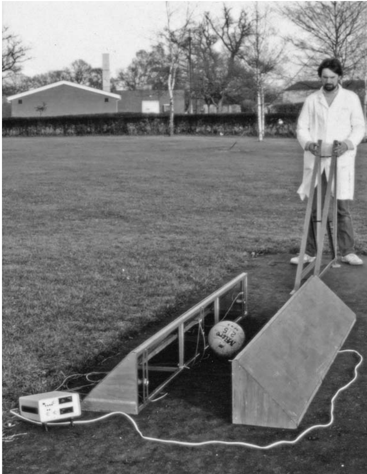
Figure 13.1 Measuring ball-rolling resistance on site
