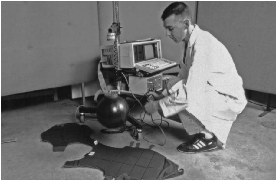
Figure 8.2 Impact resistance of equestrian jackets
