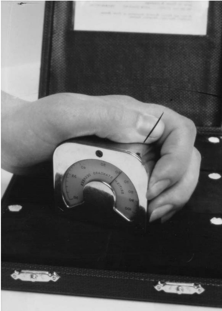
Figure 12.2 My 1949 prototype international rubber hardness degrees (IRHD) durometer is still in good working order but the calibration certificate is out of date
