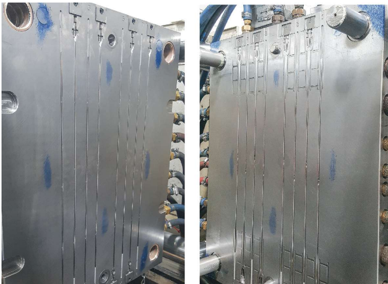
A high-volume hot-runner mold with both sides cut directly into pre-hardened plates..
