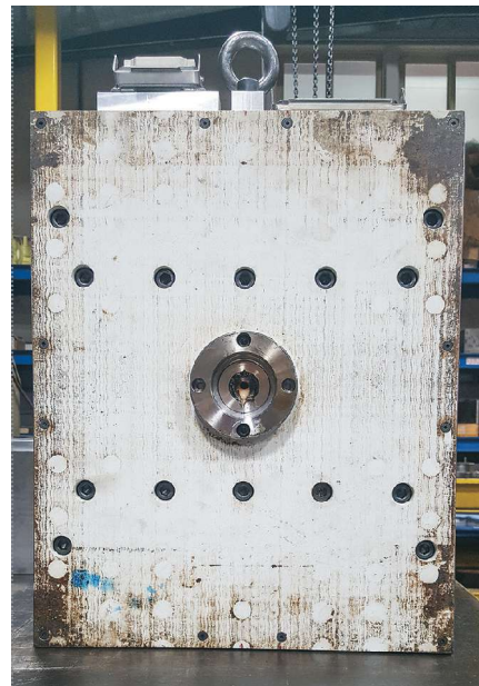
The rust marks on just the corners of this insulator plate suggest the molding machine's stationary platen is concave from wear.
