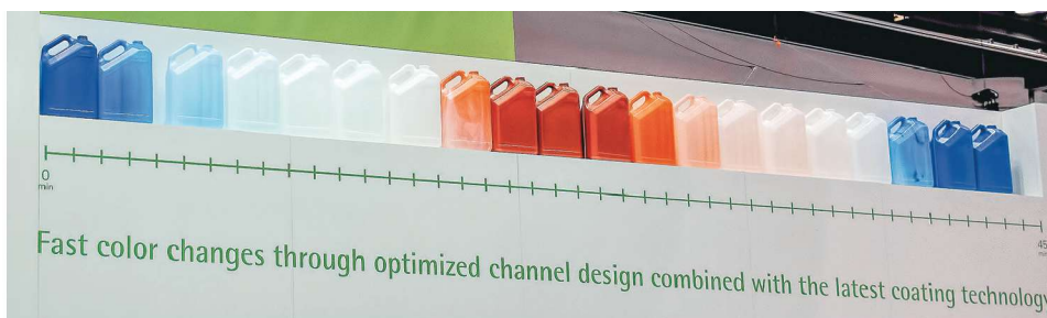
New plasma metal coating of flow channels in W. Mueller's extrusion blow molding heads allows as much as 40% faster color changes at modest extra cost.
