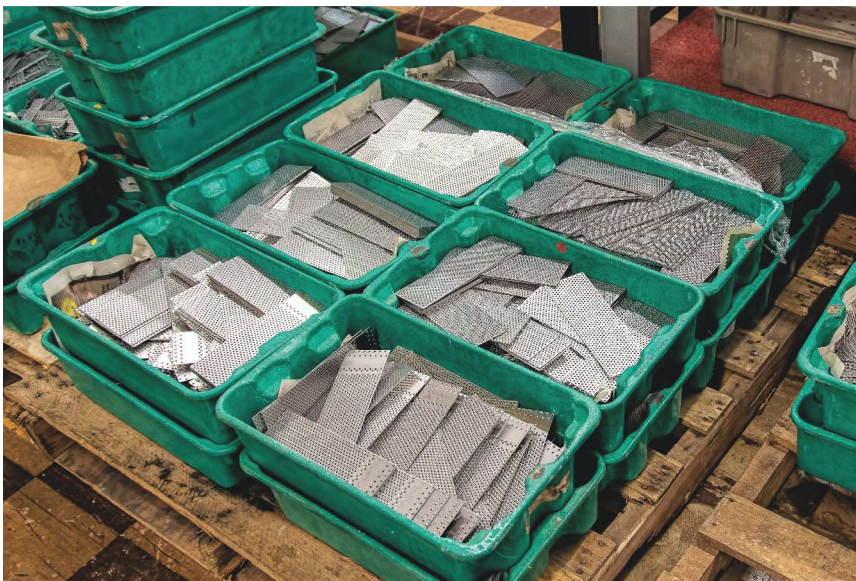
Diamond-plated metal inserts ready for overmolding with a glass-filled PC backing.
