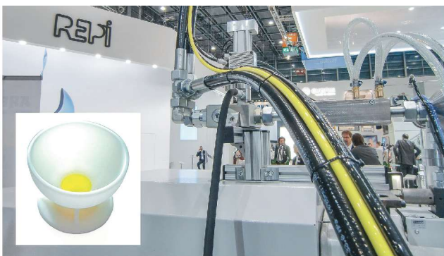
Two-color LSR egg cup was molded at Sigma Plastic Services booth using a single-barrel Arburg injection press and a single Elmet pumping system. T-coupling visible here diverted a small stream of LSR to a second static mixer and pneumatic piston pump, where the second color was added.
