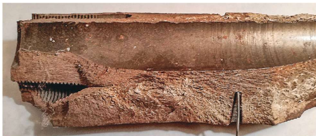
Shown here is the front zone of an injection molding machine barrel blown apart by resin decomposition gases.
