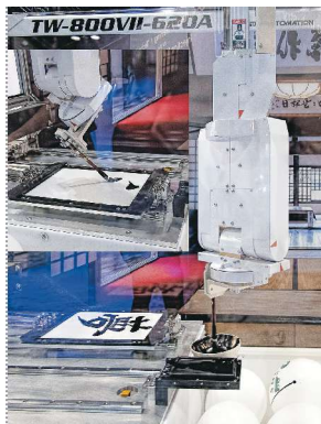
Star Automation programmed a servo robot to paint Japanese calligraphy (inset) after carefully loading the brush with ink and rinsing the brush between demonstrations.
