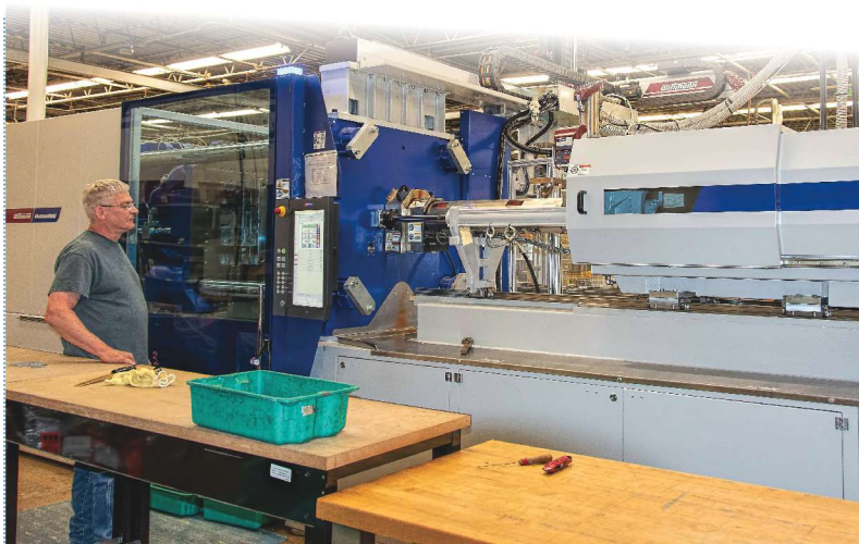
Bob Parkhurst at the Unilog B8 control of a new Wittmann Battenfeld EcoPower 300 electric press. One feature of Wittmann 4.0 enables Wittmann service personnel to access the controller remotely to diagnose problems without waiting for a technician to visit the plant.
