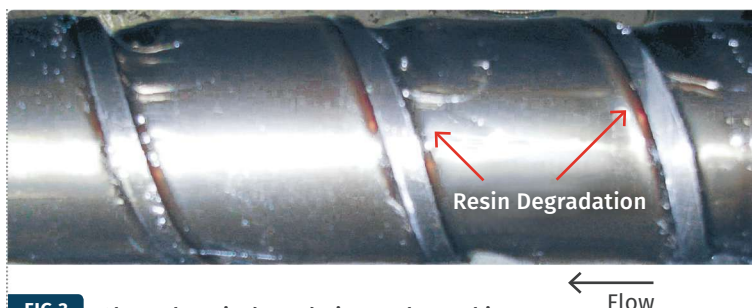
FIG 3 Shown here is degradation at the pushing and trailing flights of a screw running LLDPE.
