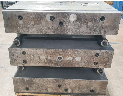
Spacer blocks on the back of a mold solve a minimum stack-height problem.
