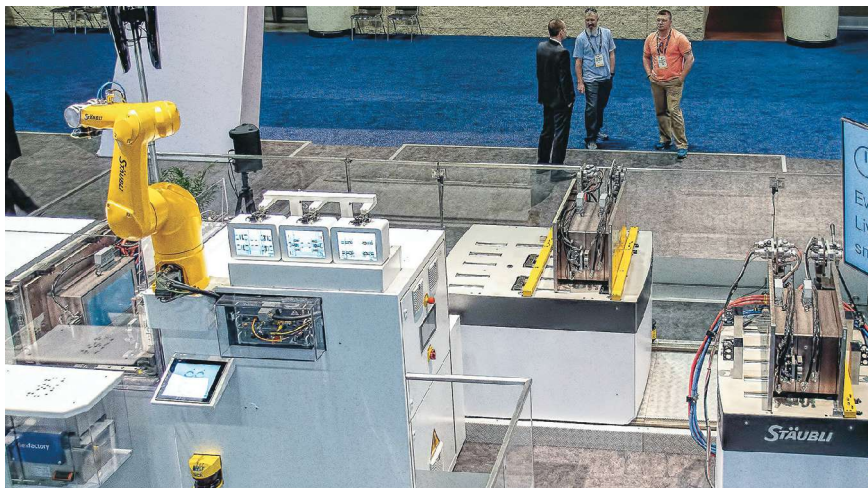
Staubli demonstrated one-minute automated mold change, using a mold preheating station (far right) and rail-guided mold cart (center). Six-axis robot (left) executed automatic change of EOAT coordinated with the new mold.
