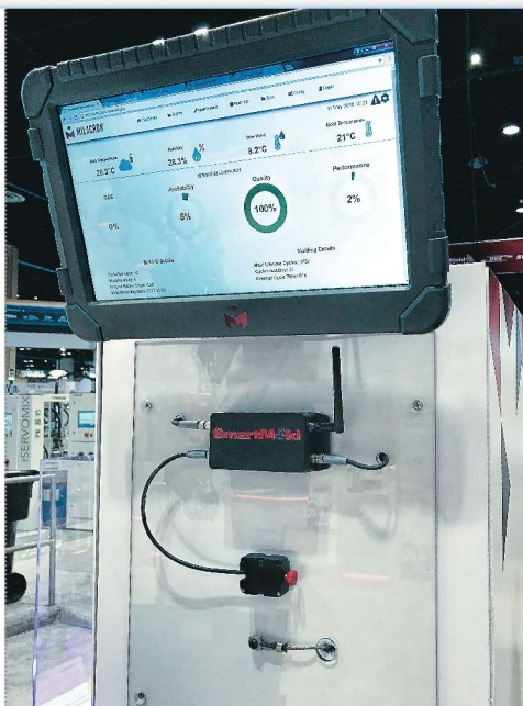
Milacron's SmartMold technology tracks key process data from the tool, including lifetime cycles, cycles in the last 24 hr, average cycle time, and more.
