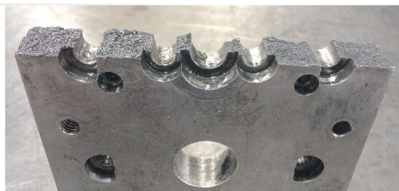
An ejector retainer plate can crack when subjected to an uneven load.
