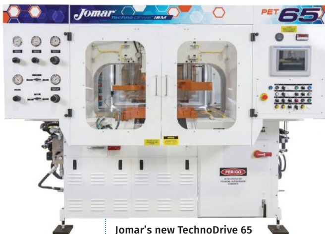
Jomar's new TechnoDrive 65 PET injection-blow machine is its first aimed specifically at non-stretched PET bottles, vials and jars.
