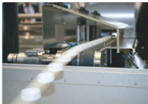
Sumitomo (SHI) Demag has cut energy consumption of its hybrid EI-Exis SP packaging machine by up to 20%, while it can still mold water-bottle caps in 72 cavities at 130,000/hr.
