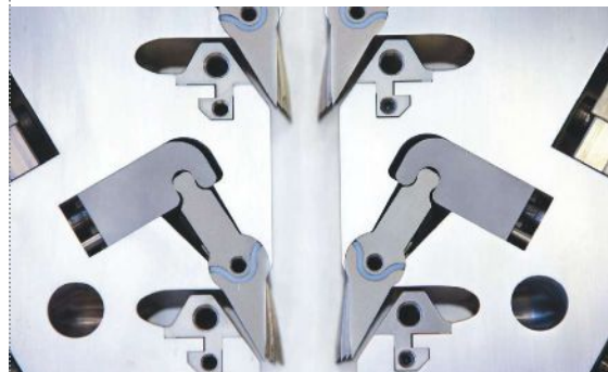
Reifenhauer's REIcofeed-Pro feedblock allows material streams to be adjusted automatically during operation.
