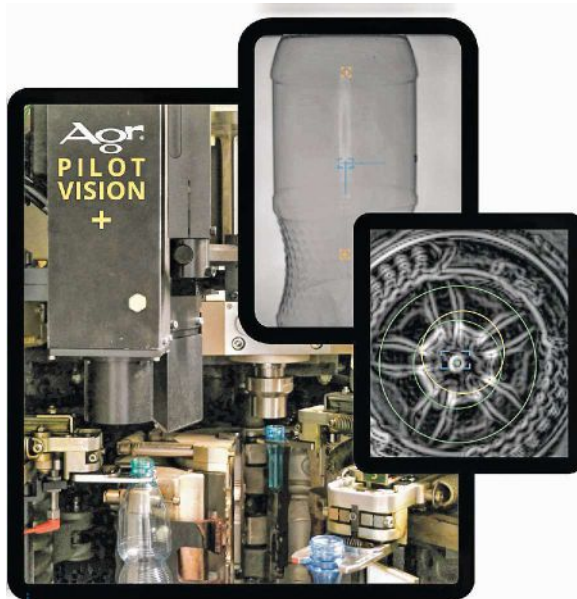
Agr’s new Pilot Vision+ provides enhanced PET-bottle defect detection with up to six cameras—including color sensing—which can be especially helpful in processing high levels of recycled PET.
