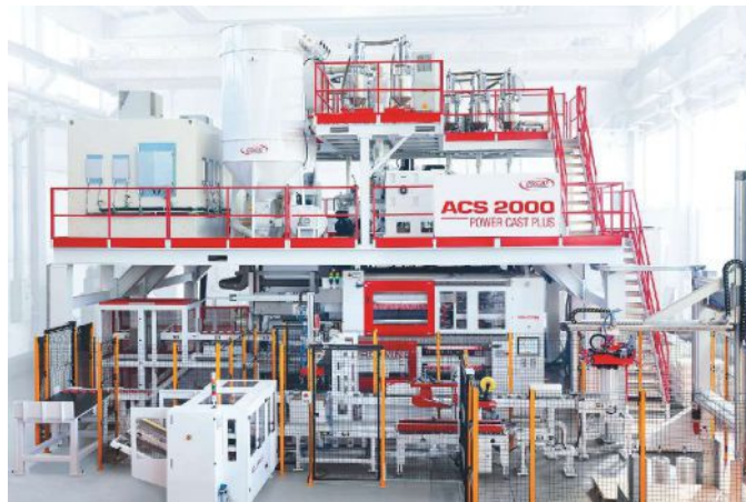
Amut will be running an ACS 2000 cast line for stretch film. The line on display will feature five extruders in a seven-layer configuration.
