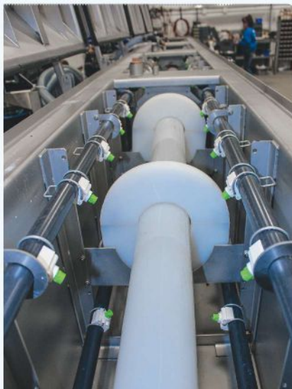
The open lid of a vacuum-sizing tank shows a larger-diam. pipe passing through guides made of UHMW-PE, a material chosen for its lubricity. The guides prevent sagging and aid in size control as the pipe undergoes vacuum sizing and spray cooling.
