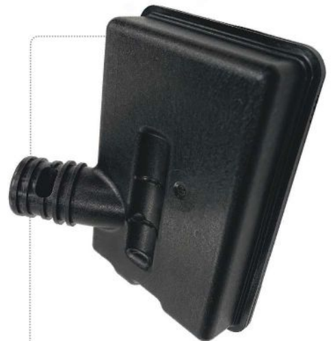
ITW Powertrain says the biggest advantage in using the ultrasonic welders is the ability to perform two different weld processes via a two-stage weld side by side. Photo shows ITW Powertrain's completely assembled auto transmission filter made of glass-filled nylon 66.
