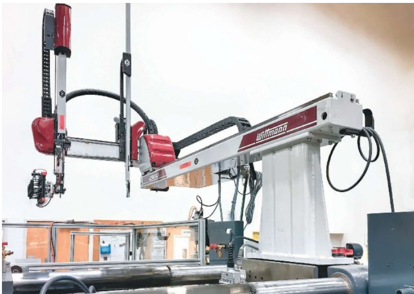
Dual-arm Wittmann Battenfeld W818S is one of the newer additions at R&D Plastics.
